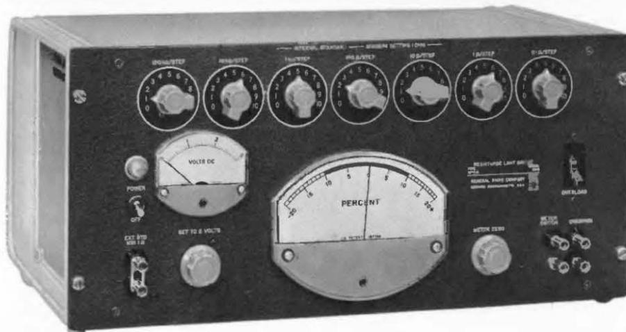
Figure 1-1. The Type 1652-A Resistance Limit Bridge.
