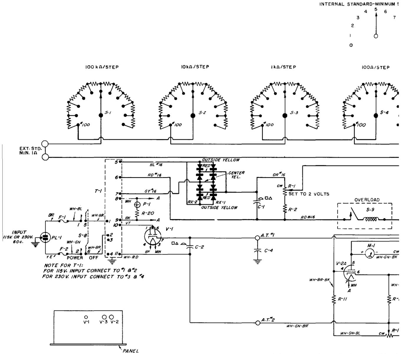
Figure 3-1. Schematic diagram for the Type 1652-A R
