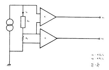
Figure 4-2. Elementary measurement circuit.
