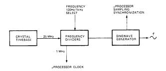
Figure 4-3. Fréquency and timing source. A pushbutton determines the frequency select function. Several clocks and synchronizing pulses as well as the measurement signal f are derived from the accurate time-base signal.
