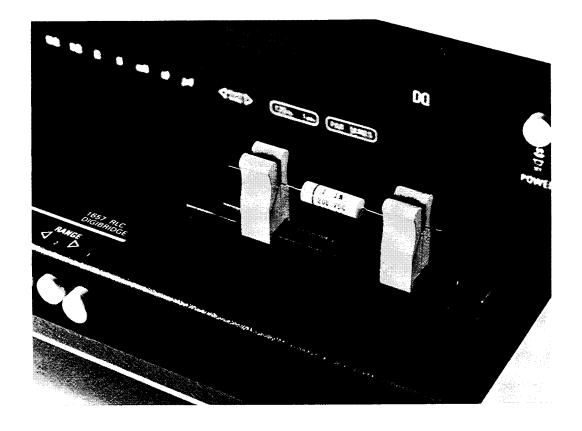
Figure 3-1. Use of the test fixture adaptors.
