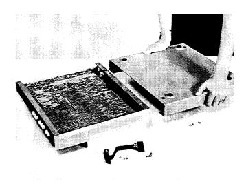
Figure 5-4. Removal of the bottom shell. The top cover has been temporarily installed as a support.
