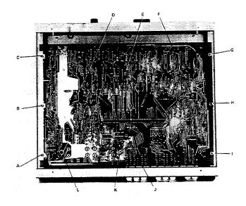
Figure 5-5. Bottom interior view. Screws ABCEGHIJ hold the C board to the chassis. Screws DF hold display-board brackets. Screws KL hold the test-fixture guide block.
