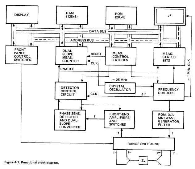
The detector control block provides sampling commands (in 4 phases). The detector is a dual-slope converter, including an integrator and comparator, which converts each phase component of the analog signal proportionally into a period of time. The dual-slope measurement is converted into a digital number by a counter that is gated by this period. From this information and manually selected criteria, the microprocessor calculates the RLC and DQ values subsequently displayed.
