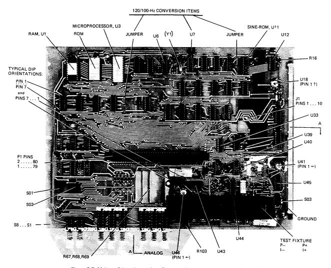
Figure 5-7. Main or C board, top view. Functional conversion between 1657-9700 and 1657-9800 involves replacement of precision oscillator (or crystal Y1, if separate) and relocation of 2 jumpers; locations indicated. Notice that DIP sockets are oriented consistently, for convenience in circuit probing. Arrows A——A indicate approximately the area of analog circuitry.
