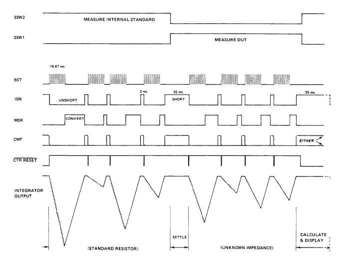
Figure 5-11. Timing diagram. One complete measurement cycle for a typical 1-kHz measurement on a 1657-9700. There are always 8 staircase cycles, one with each phase of BST for the signal from the standard (via U43 pin 8) and one with each phase of BST for the signal from the DUT (via U43 pin 1). The CMP pulses can take either a short or a long form (either is correct); the short ones are logic high for a fraction of a millisecond; the long ones are similar to ISW, but less sharp.
