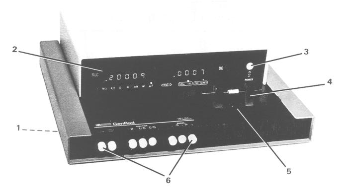
Figure 6-1. Front view showing mechanical replaceable parts.
