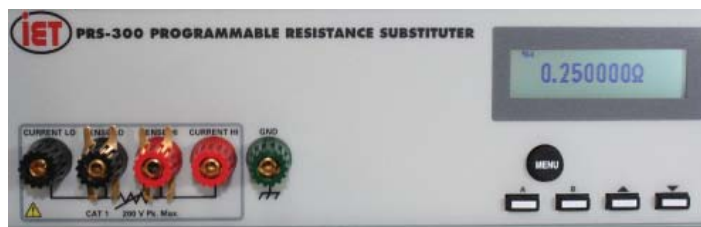
Figure 3-6 4-Terminal shorting links not connected
