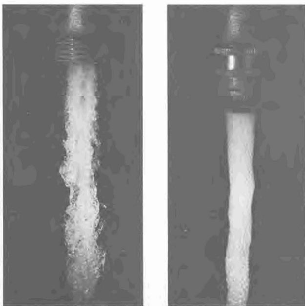
Figure 16. Single-flash photographs of a household water tap, showing the effects of a de-splash attachment. Exposures were made on Polaroid Type 47 film at f/22 with a single, high-intensity Strobotac flash.
