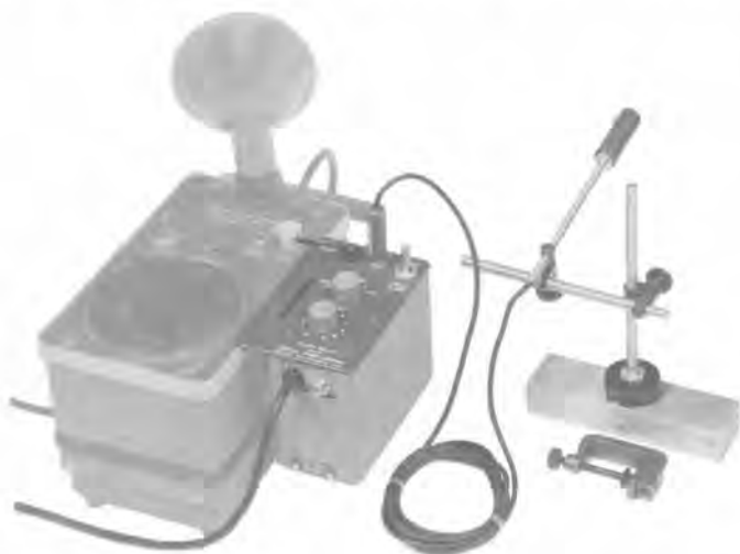
Figure 8a. The Type 1531-P2 Flash Delay and the Type 1536-A Photoelectric Pickoff shown ready for use with the Type 1531-A Strobotac electronic stroboscope.
