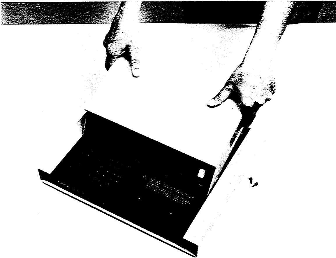
Figure 5-2. Removal of the top cover from 1692 Digibridge.
