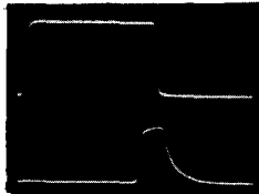
Figure 6. 6- \mu sec input, 1- \mu sec output pulses.
