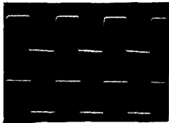
Figure 4. Square-wave modulation. The rise-and-fall time is faster in r-f output than in input.
