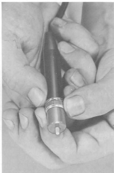
Figure 5-2. Unscrewing tip from probe. Notice little finger of hand holding cable, to withdraw inner part of probe from tip.
