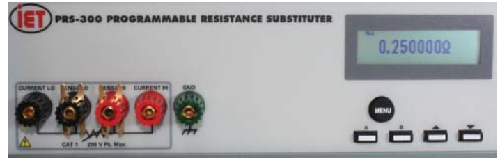
Figure 3-6 4-Terminal shorting links not connected
