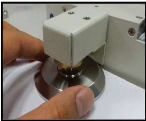
Figure 1-4 Attaching 38 mm Electrode
