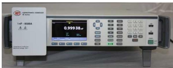
**Figure 3-7: SCA -8588A on the Fluke 8588A**
