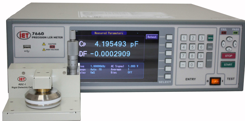
Figure 1: Connection RDC-1 Cell to 7660 Precision LCR Meter
